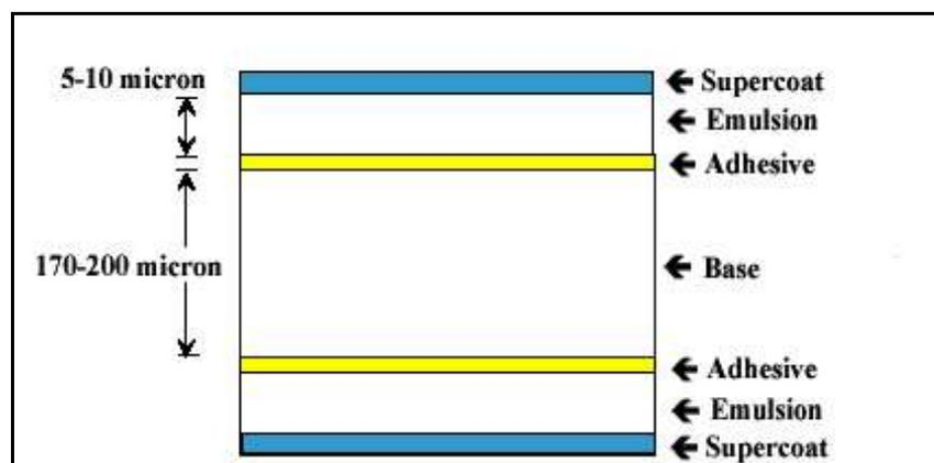
**2: Film Emulsion:** The X-ray film emulsion is composed of a mixture of gelatin (*derived from cadaver bones*) and small silver halide crystals (*grains*). The gelatin serves as a matrix which keeps the silver halide grains well dispersed and prevents their clumping. The developing and
