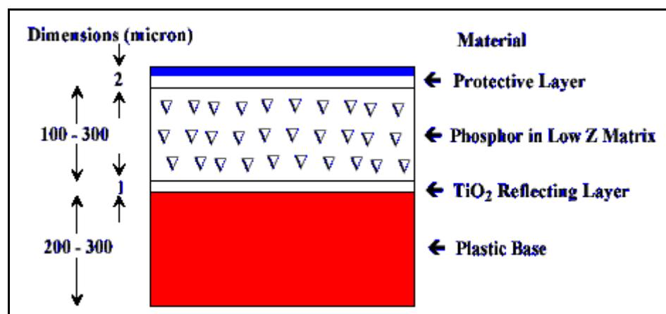
2. **Substratum:** It is the bonding layer between the base & the phosphor layer. It may be reflective, absorptive or transparent in nature.
